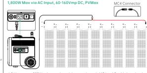
4-9 Vanpowers 200W solar panels, serial connection only,MC4 to AC cable is optional
