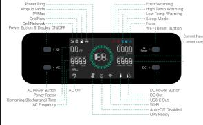
\* To activate or deactivate the cell network connection, press and hold the DC button
