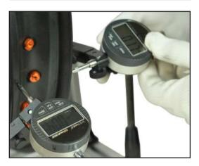
**Step 10.** Move and adjust the digital gauge pointers toward the back and surface of rim, screw down the turn-knob of the brackets. Now you are ready to truing wheels.
