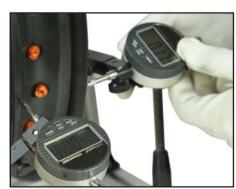
**Step 9.** Move and adjust the digital indicator pointers toward the rim back and side surface, screw down the turn-knob of the brackets. Now you are ready to truing wheels.
