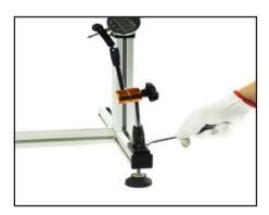
**Step 8.** Lock the bolt on the bottom of bracket
