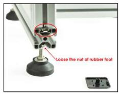
**Step 4.** Put the clip of the support bottom to the "U" slot on the stand base, than slide the clip to the center of stand base. If the clip bolt head was stopped by the bolt of rubber foot, Loose the nut
