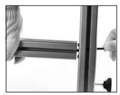
**Step 5.** Slide the clip to the center of stand base till the center hole of stand base(on the bottom) line up the clip bolt
