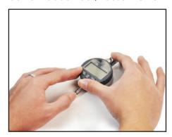
**Step 7.** Put cell button battery(LR44) into digital indicators than push the "on/off" button on the screen
