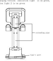
2. Put the wireless charging phones or earphone charging case on the wireless charging stand, now it is charging mode: single charging version: indication light 1 is off, indication light 2 is on blue dual charging version: indication light is on blue, indication light 2 is on blue
