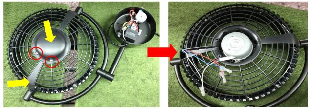
5. Loosen two screws of the motor, cut the 3 pieces close end wire connector of the motor wire, then take off motor. (Please do not cut too long in case later unable to wiring back)
