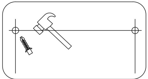
4. Hammer the expansion material into the hole
