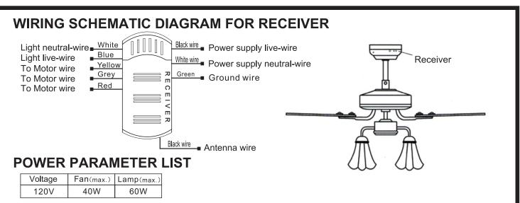
Adopt RF wireless digit emission technique, biunique controlled, coincident code rate is less than one millionth.(Emitter and receiver must be sent back to factory for maintenance if damaged.) Receiver can be controlled by any angles of the emitter in prescriptive space, unrestricted by direction. With the memory function, the controller can save the status( light and direction ) while the supply
