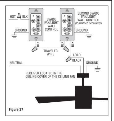
Install the First Wall Control in the Wall Box containing the "HOT" Wire.
