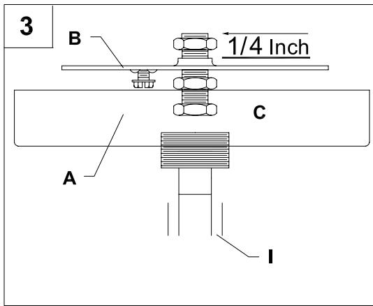
**Note:** Canopy is only needed to determine the position of the threaded nipple and fixture loop. It will be installed later.
