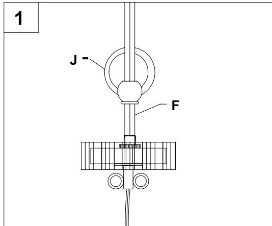
2. **Note:** The main line passes through the upper lamp body and the hanging chain connects the upper and lower lamp body.
