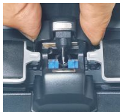
12. Put the electrode cover back then the electrode change has been done.
