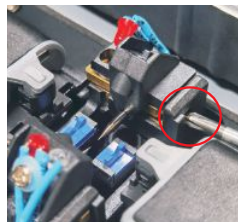
7. Push the copper gasket out of the hole, then take the electrode and the copper gasket out of the machine.
