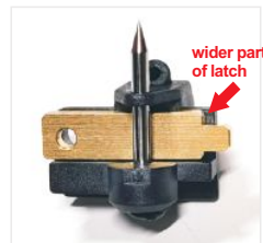
9. Replace the new electrode and put the copper gasket back to slot, please note that keep the copper gasket's wide gaps towards to the tips side.
