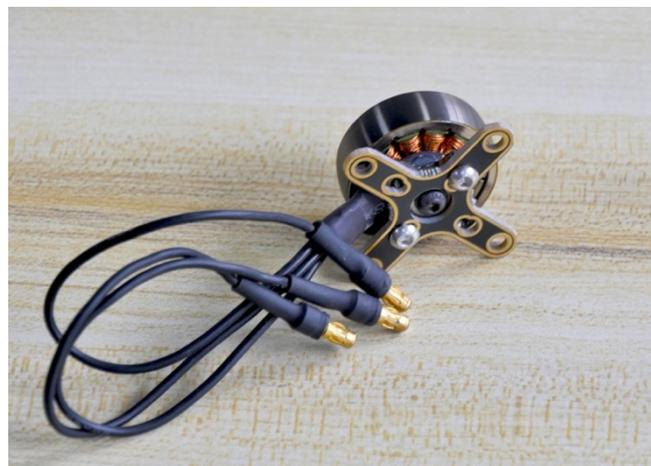
6. Install the motor, use M2.6X12 tapping screw to lock the PCB plate with motor and motor mount
