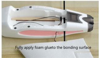
4. Glue wing-lets(Fully apply foam glue to the bonding surface, especially the front of wing-let. Adjust the bonding position and appropriate pressure to let it bond firmly)
