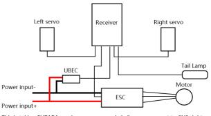
This is taking FUTABA receiver as an example.Left servo connect to CH1,right servo connect to CH6,ESC connect to CH3, UBEC and tail lamp can connect to rest any channel
