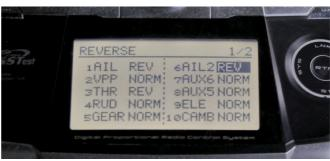
2. Power on the F-01, remove the propeller during setup. Check all Channels' movements is smooth and direction are correct.
