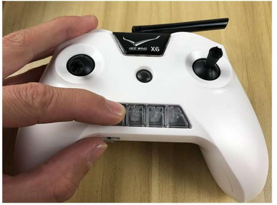
Connected with S.BUS receiver, transmitter set to regular "AIRPLANE" mode type. Find and switch on the CH5(Throttle lock) CH6 (MODE switch ) and CH7(Sensitivity), bind the transmitter with receiver. (Binding method please refer to transmitter manual)
