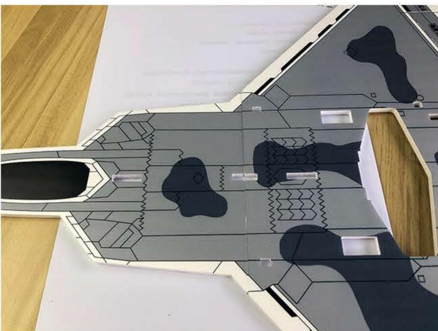
4. Find the No.7 board, cut along the connecting side.( As shown below) Bond the surface and notice to adjust the position for align. ( Note: the motor position, make sure the cross position is aligned properly when install )
