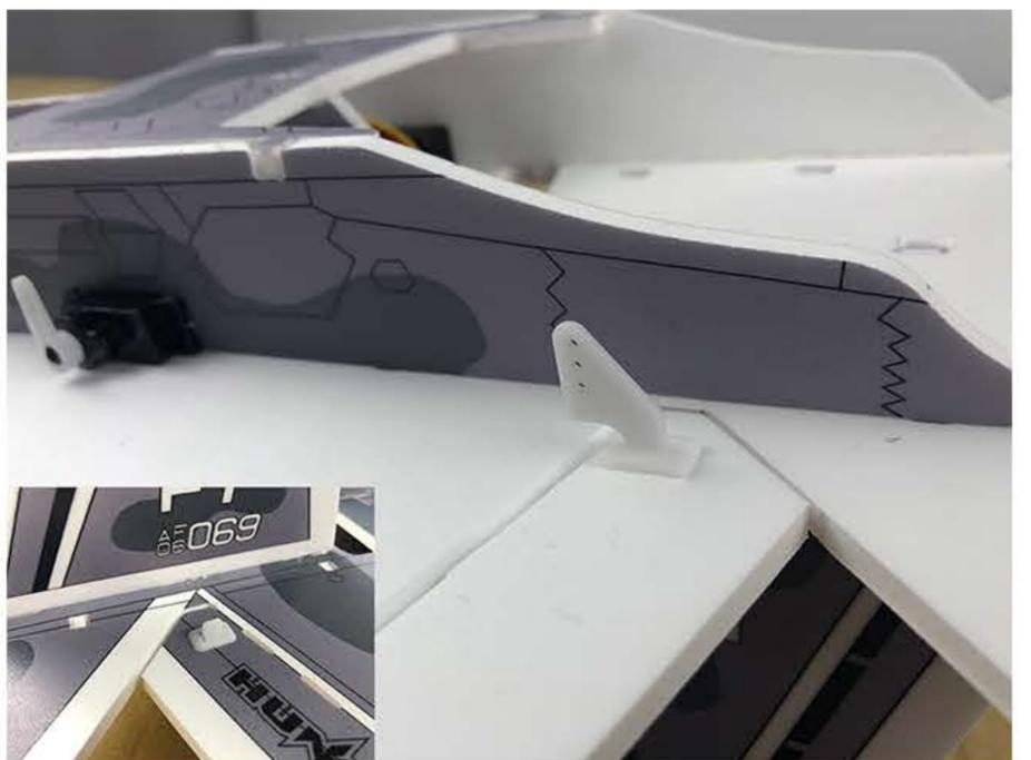
Use the rudder surface fixing seat to level fix( remove after installation), use the 65mm linkage to connect aileron and horizontal tail.( Linkage lock install to the first hole of the nylon horn). Then use 105mm linkage to connect servo and aileron.( Linkage connect to the first hold of servo arm and lock install to the second hole of aileron horn). Use the same way to install the other side.
