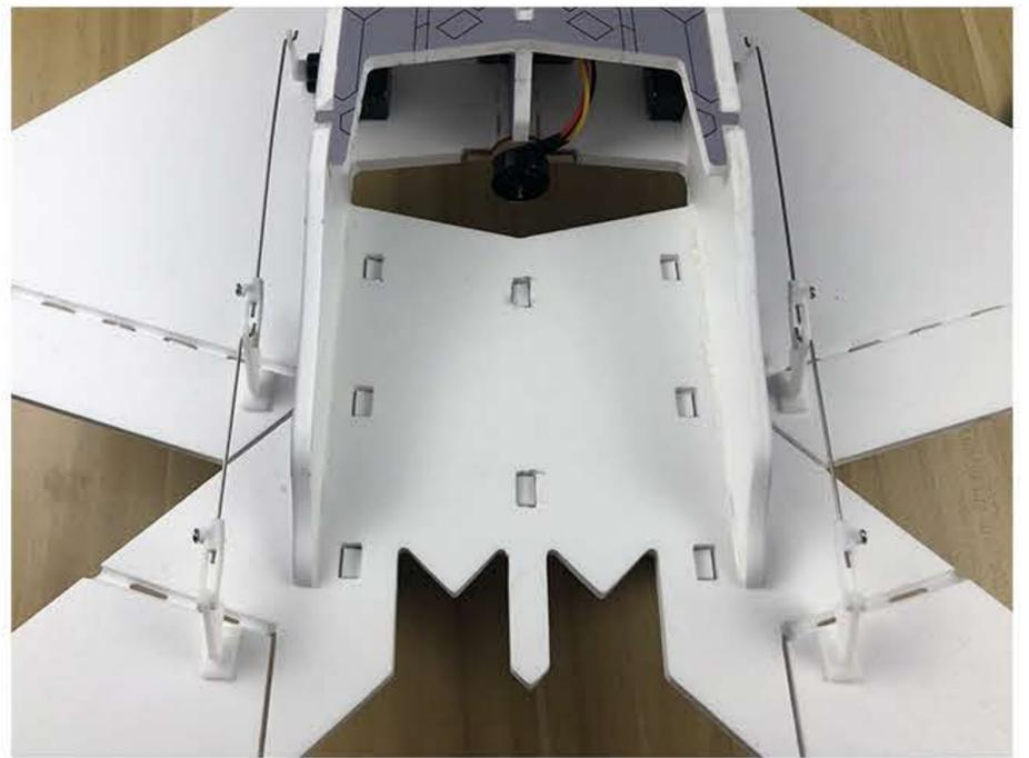
3. After installation, test the movement direction, check the flight controller correction is in properly direction. (As shown below is taking left hand throttle for example)
