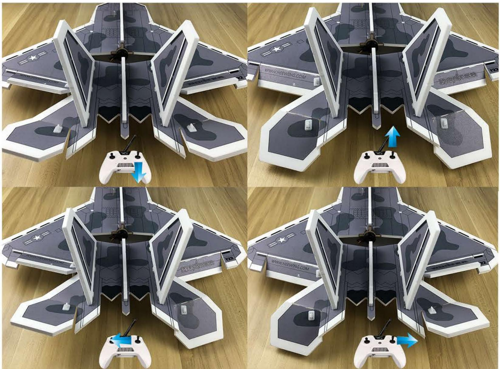
As shown below is flight controller correct direction:
