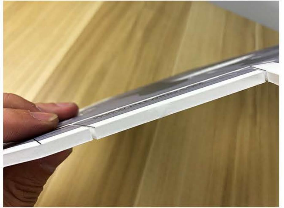
3. Find the No.2 board, cut along the connecting side. As shown below, use foam glue or hot melt glue to bond ( The red color point ) all of the following bonding are the same operate , make sure you already aligned position before glue.(You can lay flat the board on the table after bonding, use a weight thing to secure and avoid uneven bonding, influence flight) Wait for glue dry to do the nest step.
