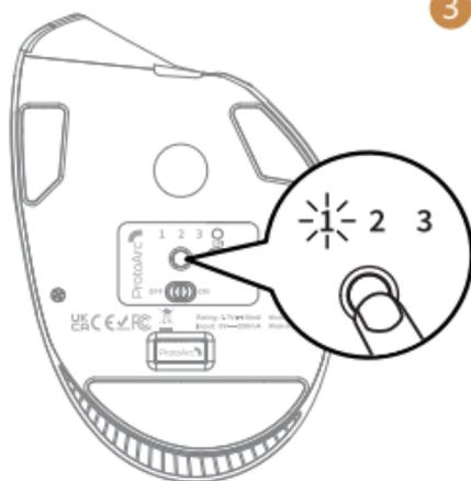
3. Press the channel switch button until the white light 1 is on and enter 2.4G USB channel.
