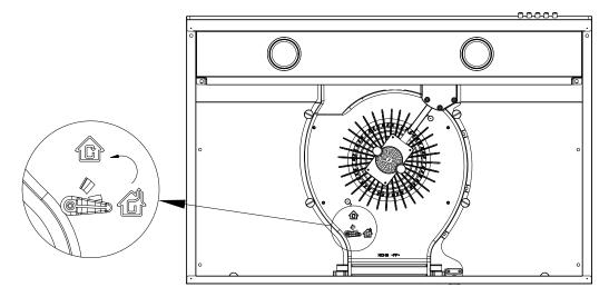
• Outdoor exhausting: Turn the adjuster to outdoor position, install the outlet, turn on the range hood, then the air will be vented from the outside outlet.
