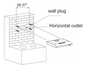
4) Lock the lower two holes with 0.16"\*1.18" screws.
