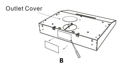
3) Install the air outlet assembly on the circular air outlet at the back of the range hood;
