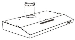
4) Align the air ventilation port of the range hood with the cabinet ventilation hole at the bottom, pass the power cord through the power hole, and then use four 0.16"\*1.18" screws to lock into the corresponding position of the pencil marked in the cabinet to fix the range hood.
