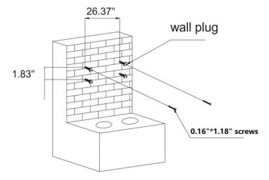
3) Put the range hood onto the top two screws, and lock the self tapping screws tight;
