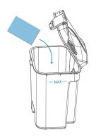
2. Fill up the clean water tank and make sure to keep the water level below the Max mark on the tank. Lift the water tank only when its cover is buckled, so as not to damage the rotating shaft
