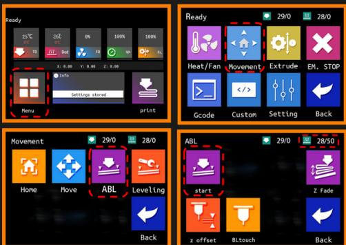
Click "Menu"→"Movement"→"ABL"→"Start" The printer will start to preheat the hotbed, and then will prepare for auto bed levelling.
