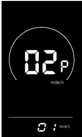
Fig. 6-2 Imperial System Setting Interface
