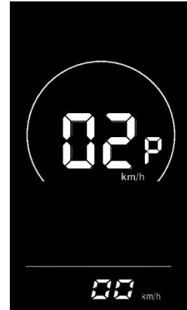
Fig. 6-3 Metric System Setting Interface
