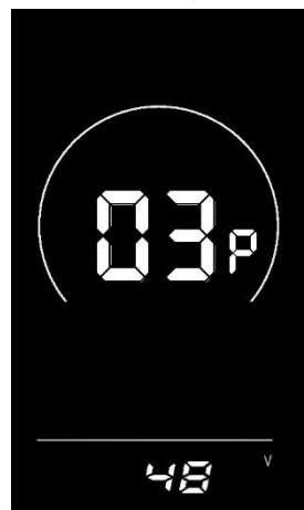
Figure 6-4 Rated voltage setting interface
