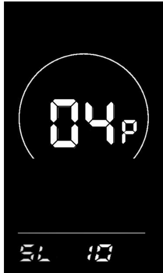
Figure 6-5 Auto Power Off Time Setting Interface
