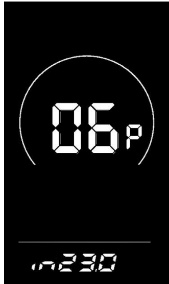
Figure 6-7 Wheel diameter setting interface
