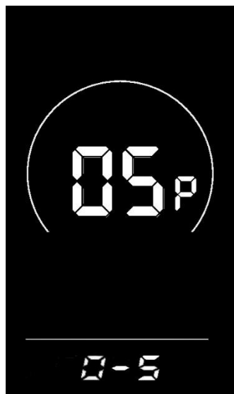
Figure 6-6 PAS level setting interface
