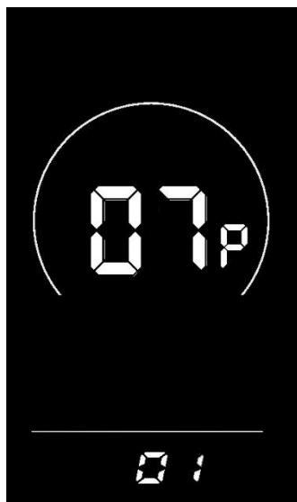
Figure 6-8 Number of speed sensor magnets setting interface
