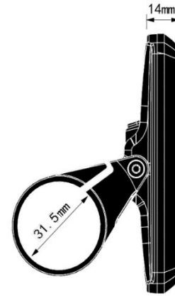
Fig. 3-4 Side View of Display 80C Dimensions
