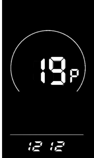
Figure 6-22 Power-on password setting interface
