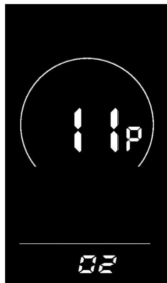
Figure 6-12 Pedal assist sensitivity setting interface
