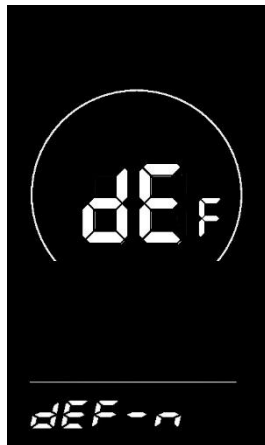
Figure 7-1 Restore Factory Default Settings Interface
