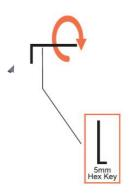
(2) The mudguard support shall be aligned with the front fork mudguard take-up hole position, and then threaded into the screw for tightening.
