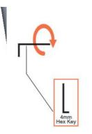
(2) Install 4mm hexagon wrench clockwise. Do not tighten the 4 bolts in FIG. A. Adjust the handle to the proper Angle in Fig. B, and then tighten the 4 bolts with proper force.
