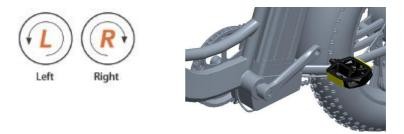
(2) Tighten the right pedal "R" clockwise, Tighten the left pedal "L" counterclockwise.
