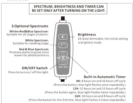
**Note:** 1. When the blue signal light under the timer icon is on before you press the ON/OFF button, it indicates the whole light is powered on.
