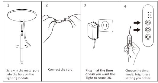
**Note:** To change the timer mode or change the time of day when the light turns on, please plug out for 15 seconds and above, and then plug in at the time you want it to turn on and select the timer mode you prefer. Then the light will come ON at the time each day.
