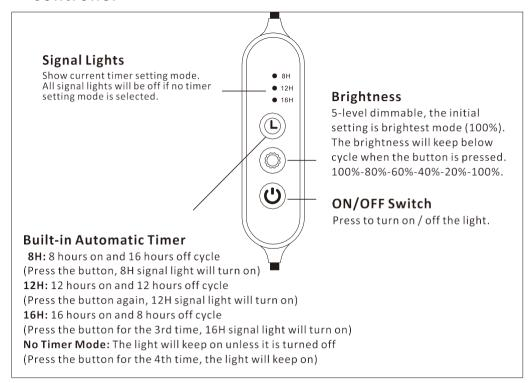
**Note:** 1. The initial setting of this light is 100% brightness and no timer setting mode is selected.
