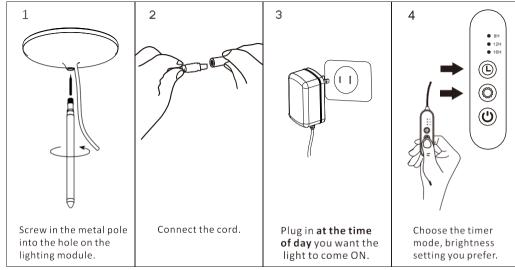
**Note:** To change the time of day when the light turns on, please plug out for 15 seconds and above, and then plug in at the time you want it to turn on. Then the light will come ON at the time each day. Please kindly note this is the ONLY way to change the time of day when the light turns on.
