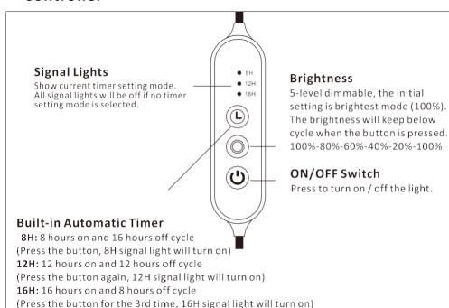
**Note:** 1. The initial setting of this light is 100% brightness and no timer setting mode is selected. The light will keep on for 24 hours if you don't choose any timer mode after you turn on the light.
