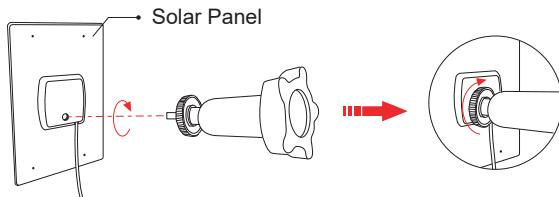
4.Screw the locking screw cap into the base. Make sure that the universal joint is angled upward.
