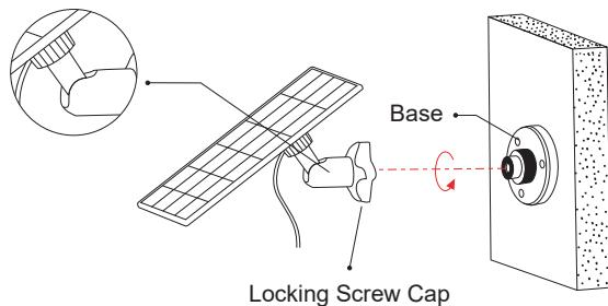
5.When adjusting the solar panel left or right, loosen the locking screw cap, turn the sleeve rod, and retighten the locking screw cap when the panel is in the desired position.
