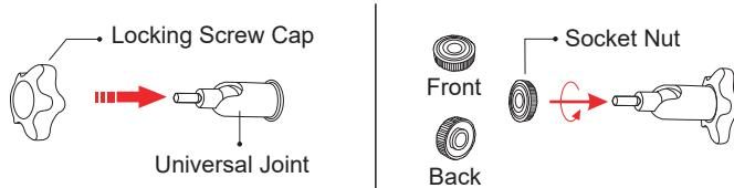
3. Screw the universal joint into the back of the solar panel. Tighten it firmly with the attached nut.
