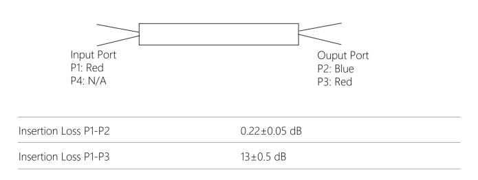
Order notes to our customers: The default parameters are as follows. For special needs, please contact sales. 1) Connector FC/APC, 900 um, 1 m by default for all devices except for high power devices. 2) Slow axis working, fast axis blocked, connector key is aligned to slow axis by default for PM devices.
