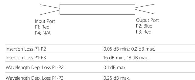
Order notes to our customers: The default parameters are as follows. For special needs, please contact sales. 1) Connector FC/APC, 900 um, 1 m by default for all devices except for high power devices. 2) Slow axis working, fast axis blocked, connector key is aligned to slow axis by default for PM devices.
