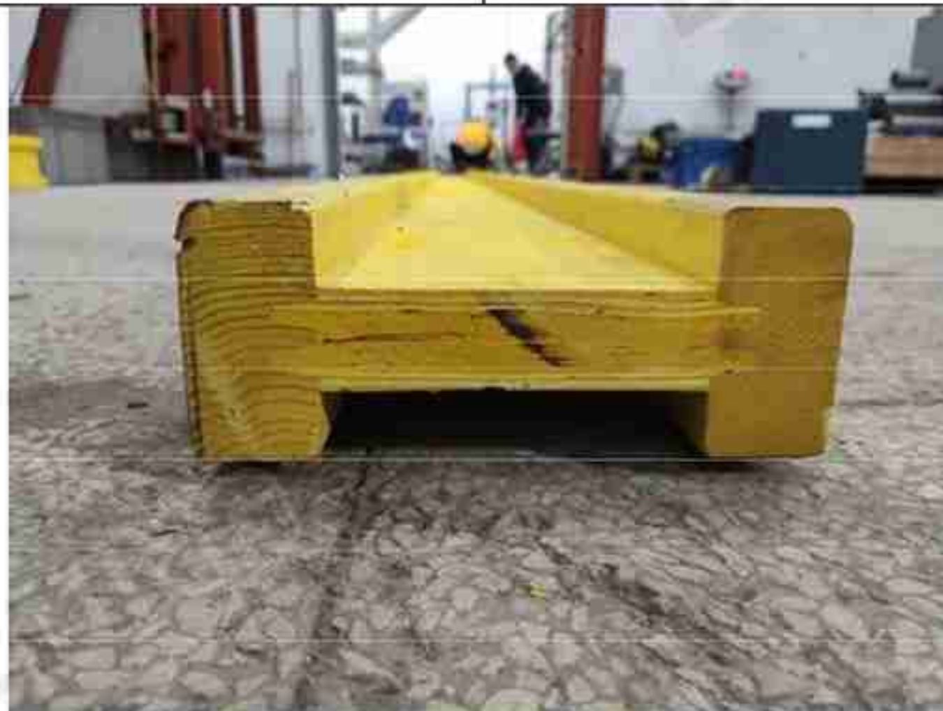
Bending Resistance - Section View
