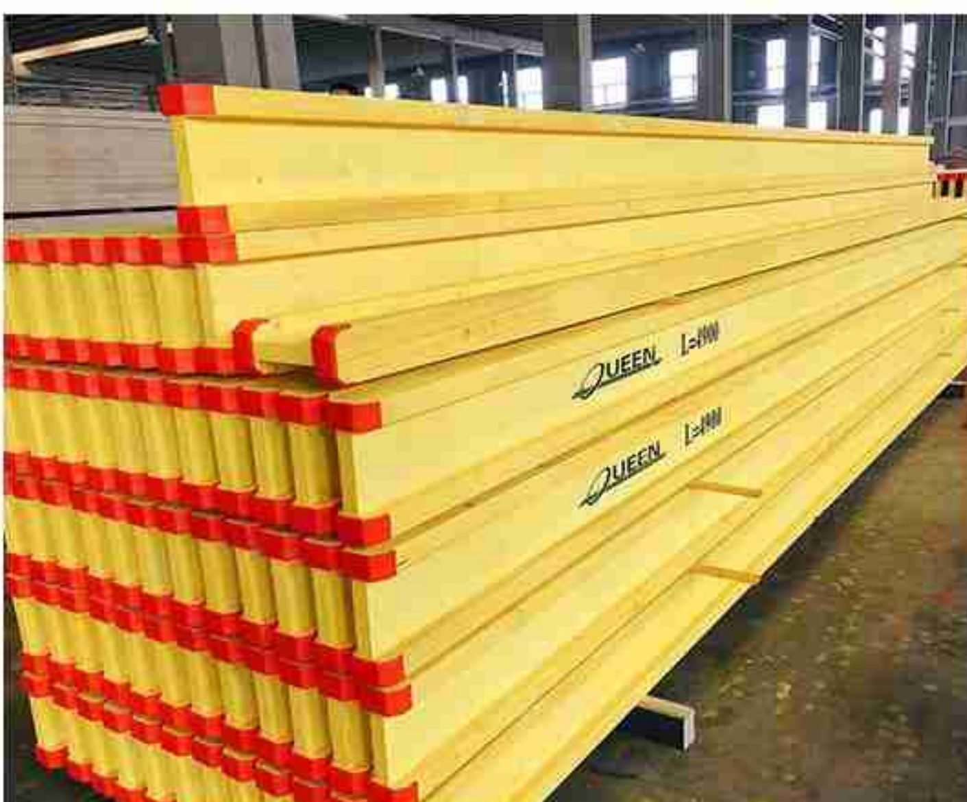
H20 Beam Workshop
