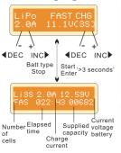
Charging current will become lower when it progress to the end of charging. Aspecific CV process will be reduced to end the charging process earlier. In fact, the charging current will goes to 1/5 when the charging process comes to 1/10. Charging capacity will be a little smaller than normal charging, but charging time will be shortened accordingly.
