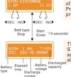
Set charge current on the left and the final voltage on the right. Range of the charge current is 0.1-1.0A; range of final voltage is 0.1-25.0V. Press START/ENTER key for more than 3 seconds to start the program.
