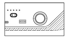
• Power ON/OFF: Long press the power button to turn ON/OFF the unit, the led indicator will light up/off.
