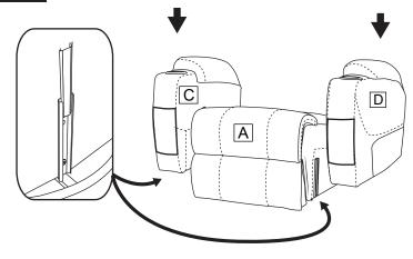
Insert two armrests to the chair base, make sure the slots on the armrests fully assembled to the bottom part.
