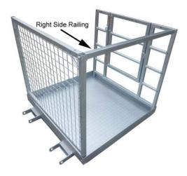
Assemble the Right Side Railing and Left Side Railing onto the Front Railing and loosely bolt in place. Line up the holes with the mating holes of the Rear Railing and loosely bolt in place utilizing the lower hole only.
