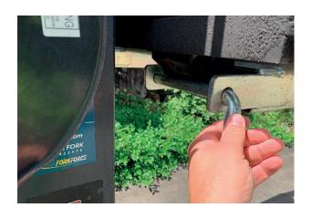
Insert the locking pin through both plates and repeat on the other side as shown in Figure 3.
