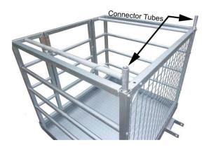
Place the Connector Tubes into each of the Rear Railing posts as shown, hold in place by bolting thorugh the appropriate side railing, the rear railing corner posts and the connector tubes.
