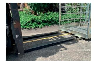
Install the F-WP-N working platform to the forklift, move the forks to the correct width, and insert the both forks into the pocket as shown in Figure 1.
