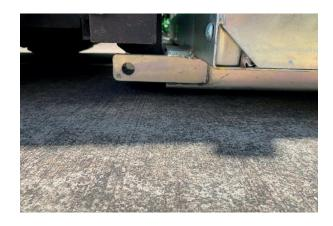
Drive the forklift forward until the back of the working platform is firmly against the fork lever or fork radius as shown in Figure 2.
