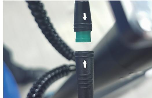
When connecting these two connectors, the arrow must be aligned with the arrow. You can turn on the power only when the assembly is completed.
