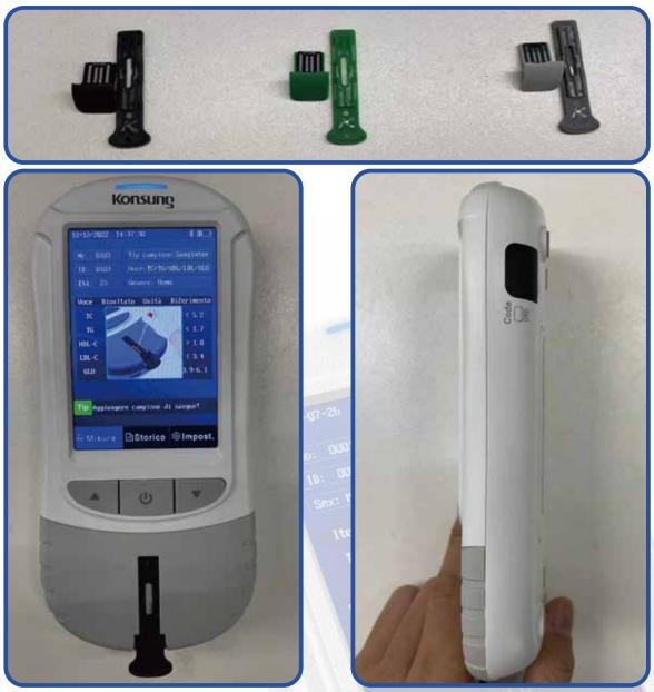
2. Ensure that the batch number and model number on the code card are the same as the test card packaging when using. New kits are supplied with new code cards, do not reuse them.
