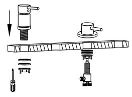
6. Pulling pipe connect with the conversion A through the shower holder. Gravity ball fixed on the top of the pull out pipe. Water nozzle connect to he conversion B, switch water outlet connect to the connector C and finally contact to the hot and cold water hose.
