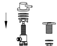
4. Fixed the switch and fasten the nut. Install the converter handle.
