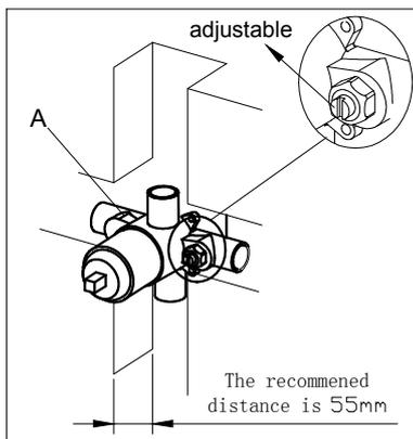
1. Fix the shower valve (A) into the wall. Use a level to ensure that the valve is straight and level. The distance between the bottom of the body and the surface of the tile is 55mm.
