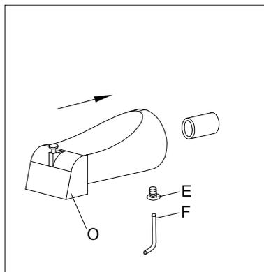
5. Turn the water on for 1 minute to flush any debris. Install the tub spout (O) into the outlet on the wall. Tighten set screws (E) with Allen key (F).
