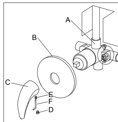
3. Remove the protective cover when the finished wall is completed and install the escutcheon (B) to the valve (A) and press it against the finished wall. Then, install the handle (C), tighten set screws (E) with Allen key (F), and put on the indication buttons (D).
