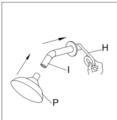
4. Turn the water on for 1 minute to flush any debris. Apply Teflon tape (H) to the threaded tail pipe and install the shower hose (I) into the outlet on the wall. Then connect the top shower (P) to the spout.
