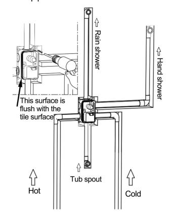
4 .Install the upper outlet pipe and the top shower head.(wrap the PTFE tape on the thread)
