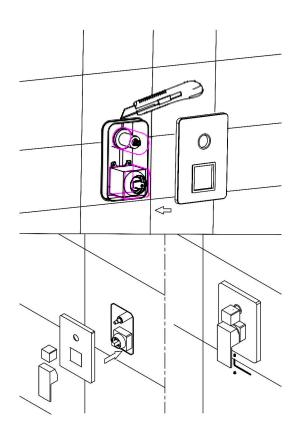
Before installing the faucet, please be sure to remove sundries and sludge from the water pipe to prevent sundries from blocking the faucet.
