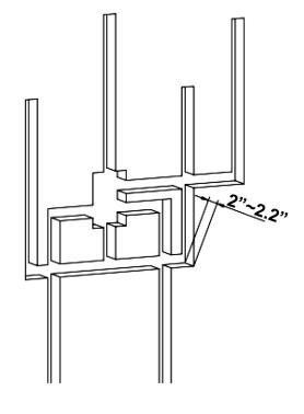
3. After fixing ceramic tiles, cut off edges of the embedded box, remove the protective cover and install the panel.
