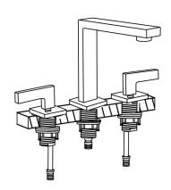
4. Connect the pipe of spout and two handles.
