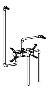
7. Install the handle according to the direction in the picture. Install upper outlet pipe and hand-held shower bracket. (wrap the PTFE tape on the thread.)
