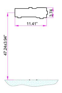
2. Chisel the wall according to the size indicated in the picture.
