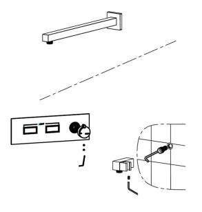
6. Ceramic tile hole 25\*8cm. Four positioning films must be closely attached to the appropriate mud. (tile + mud thickness must not exceed 2.2cm) After finishing the decoration of the ceramic tile wall, take out the cover of the embedded box and install the panel.
