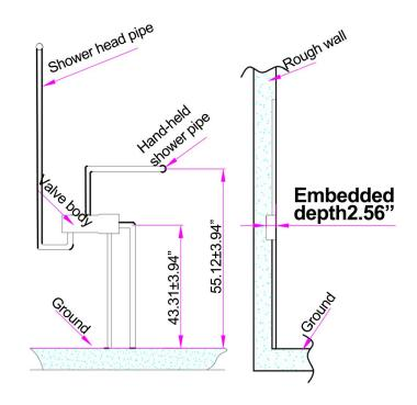
3. Connect the hot melt pipe as shown in the figure.
