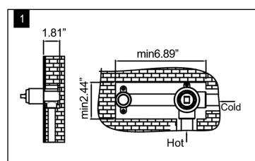
1.The wall opening Min size of the main valve body is 6.89"x2.44" and the depth is 1.81". Note: The depth dimension is the size of the tile after the wall is finished. If installing on the wall embryo, please reserve the appropriate tile thickness.
