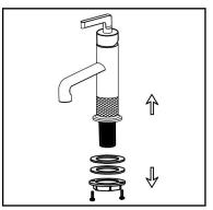
1. Remove the rubber washer, metal washer and locking nut from the faucet.
