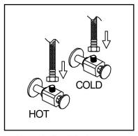
5. Attach flexible hose to water supply.
