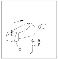
5.Turn the water on for 1 minute to flush any debris.Install the tub spout (0) into the outlet on the wall,Tighten set screws (E) with Allen key (F).
