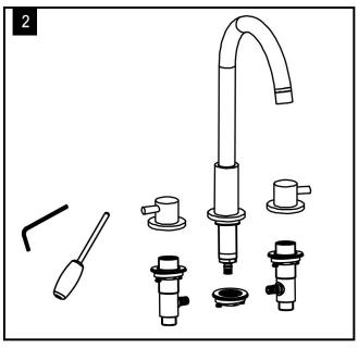
2. Use the tool to disassemble the handles and spout firstly.
