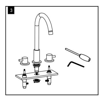
3. Put the spout and handles through the holes on the bathtub, adjust them to the proper direction and tighten them with the screws. The direction of the handles shown in the picture is closure.
