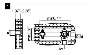
1.The wall opening Min size of the main valve body is 6.77"x2.38" and the depth is 1.97". Note: The depth dimension is the size of the tile after the wall is finished. If installing on the wall embryo, please reserve the appropriate tile thickness.
