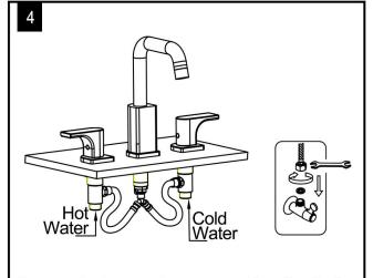
Connect the hose to the spout and handles firstly, and then connect the inlet pipes, Red hot Blue cold, connect the other end of the inlet pipes to the angle valve.
