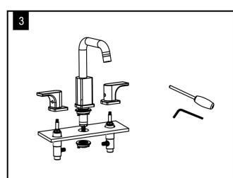
Put the spout and handles through the holes on the bathtub, adjust them to the proper direction and tighten them with the screws. The direction of the handles shown in the picture is Turn On.
