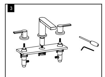
Put the spout and handles through the holes on the bathtub, adjust them to the proper direction and tighten them with the screws. The direction of the handles shown in the picture is Turn On.
