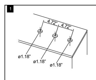
Make three holes on the side of the bathtub according to the size given in the picture above.
