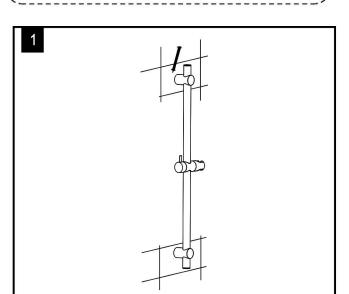
Fix the slide bar on the wall to be installed, use a
