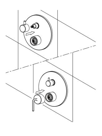
6. Mount Holder for top sprayer, outlet for top sprayer and holder for handheld sprayer. Convovle teflon taperound screw.
