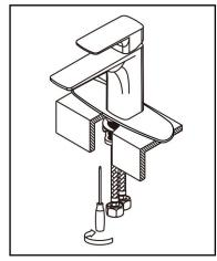
3. Use hand screw the locknut, then use cross screwdriver to screw the cross screw on the locknut, strengthen the fastness.
