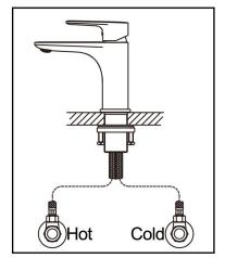
4. Connect two inlet hoses on the faucet to angle valve. Connect red inlet hose to hot water supply, and blue inlet hose to cold water supply.
