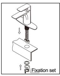
2. According the remove step screw the fixation set from the basin bottom to faucet installation base.
